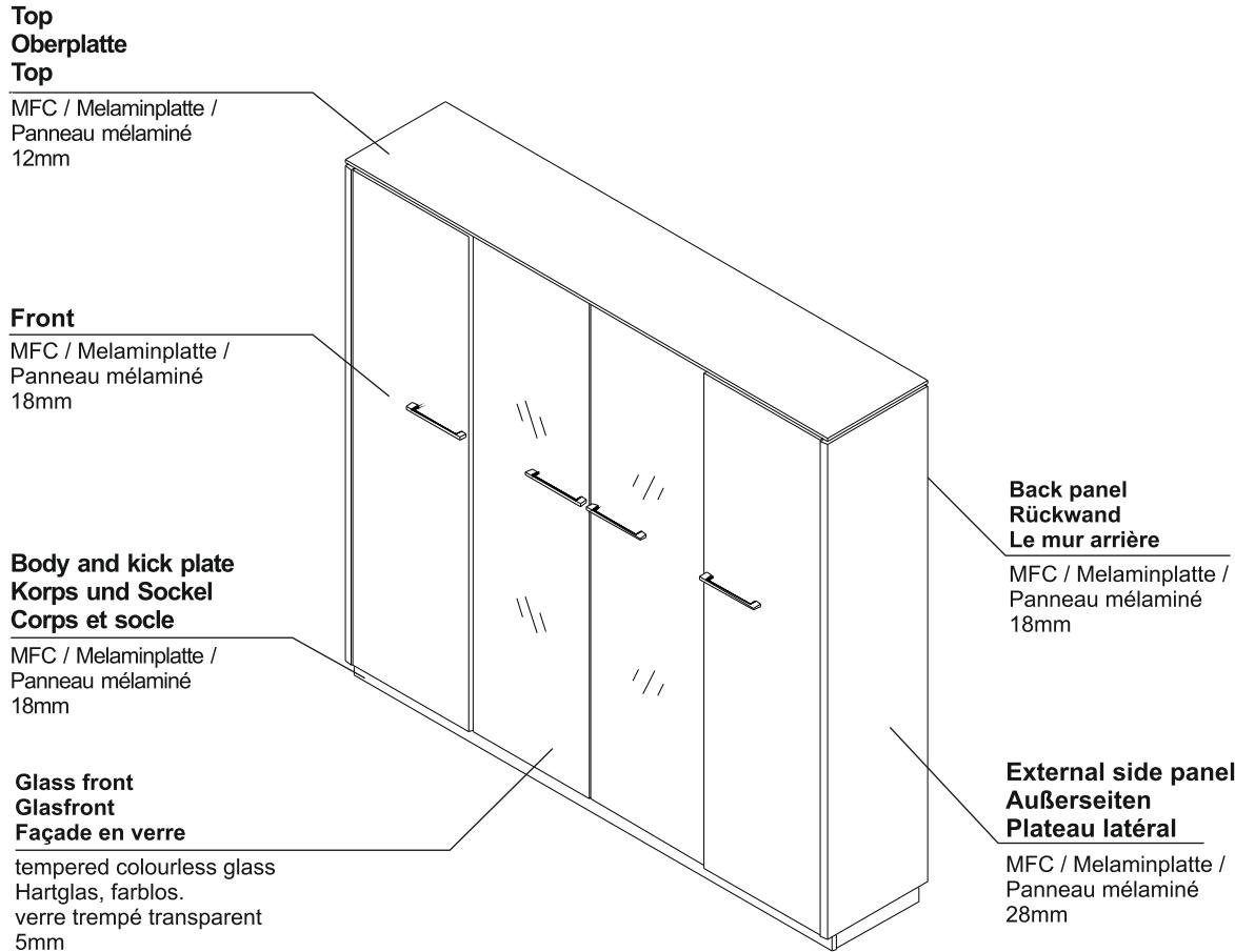
\* Cabinets do not have locks. There is a possibility of fixing two-point locks for an additional cost of 40 EUR per piece only in panel doors. In case of placing an extra order for the cabinet with lock "Z" symbol has to be added in the end product index. There is no possibility of fixing a lock in a glass doors.
